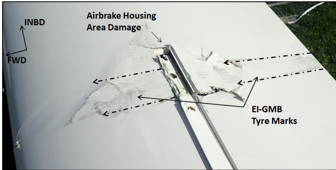
Photo No. 4: Impact point on EI-GLA port wing and damage to airbrake housing area
